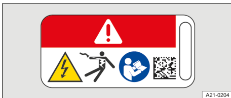
Fig. 4 Warning sign on high-voltage components.
