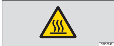
Fig. 6 Warning sign for hot surfaces on the battery charger.
