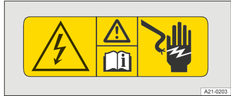
Fig. 5 Warning sign in the bonnet space.
